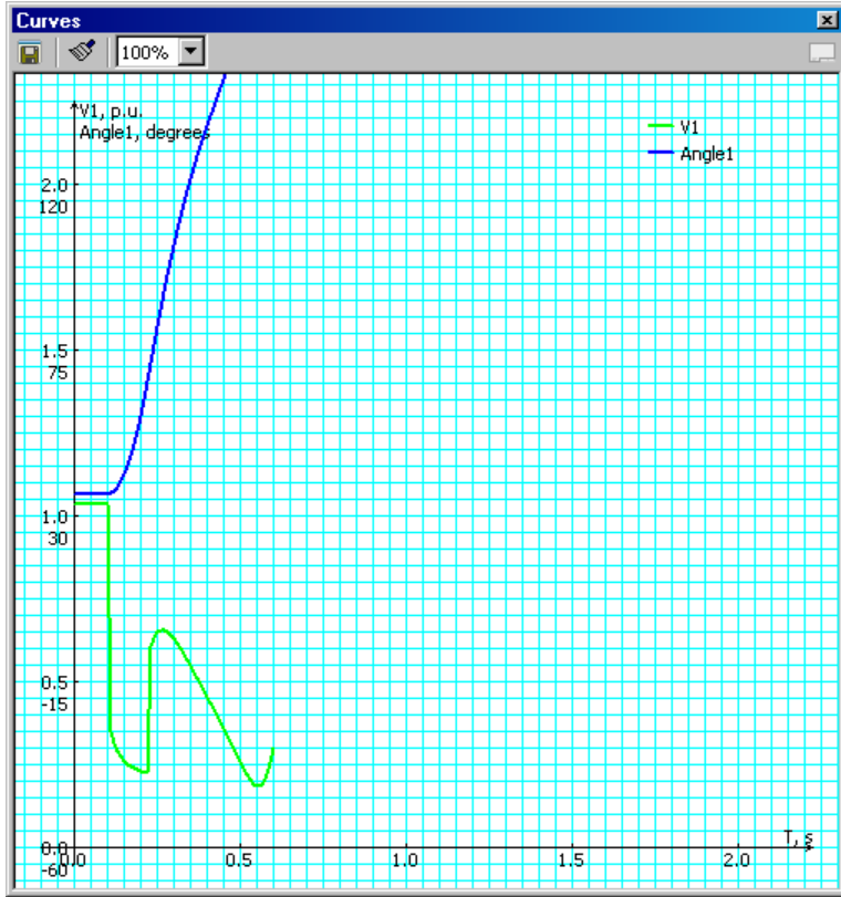
Figure 6-22. Fault at Bus # [redacted] 115.0 Clears in 0.13 sec
