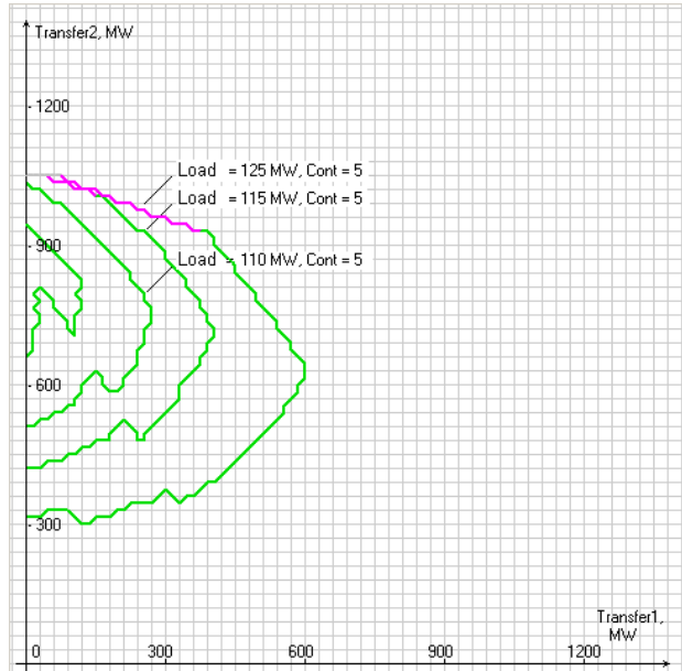
Fig. 9. Dependence of the Size of the Operating Region on the Amount of Load Curtailment (from 105 MW to 125 MW)
